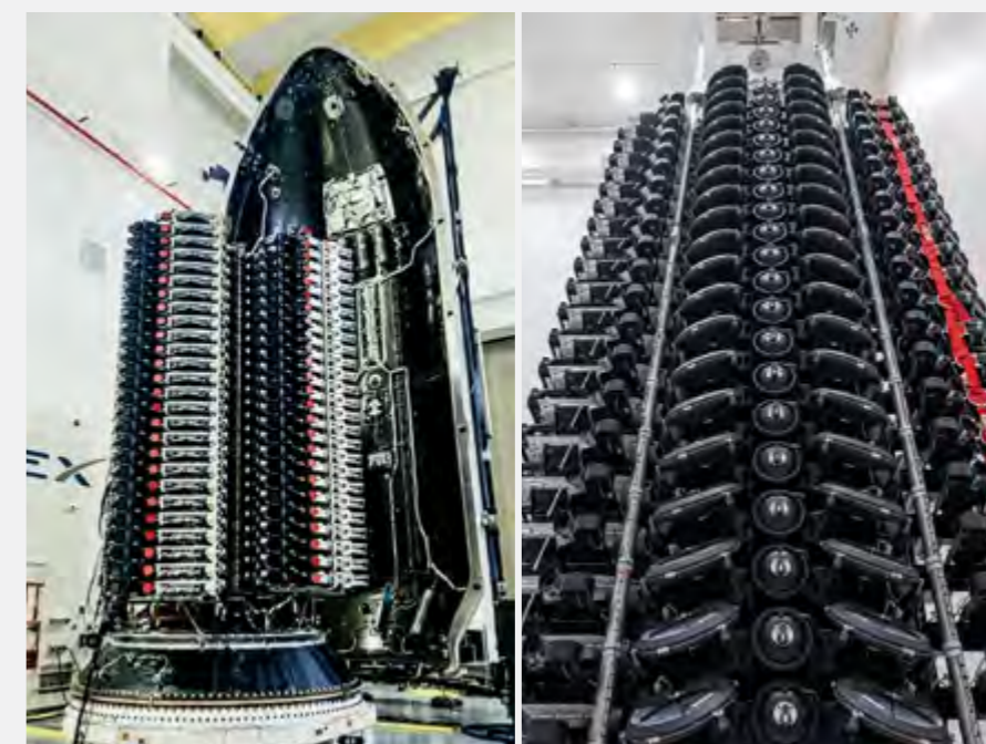
A group of 30 Starlink satellites under the fairing of the Falcon 9 launch vehicle.
