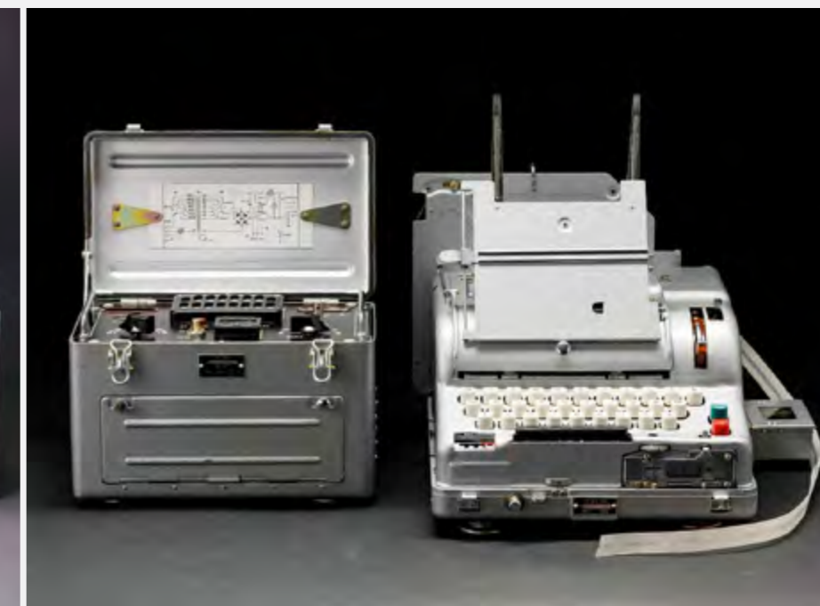
M-125-3M (“Fialka-3M”) – third version of the Soviet disk electromechanical cipher-encryption machine. © Cryptography museum
